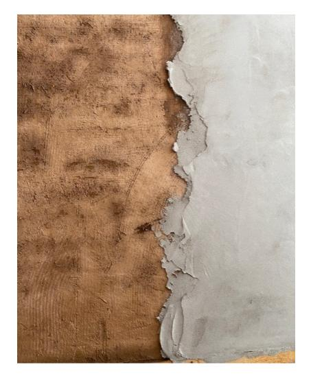
**NATURAL PLASTER** – The early straw bale houses in Ontario were plastered with cement, lime, and sand. Today recipes have mostly shelved cement in favour of clay, lime, chopped straw and sand mixes. They offer better protection from the elements, less maintenance and lower carbon emissions.
